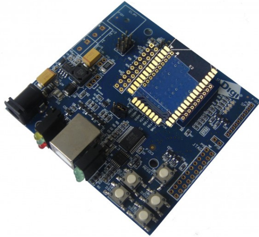
Figure 3.5: Digi XBee Development Board[Dig11b]
